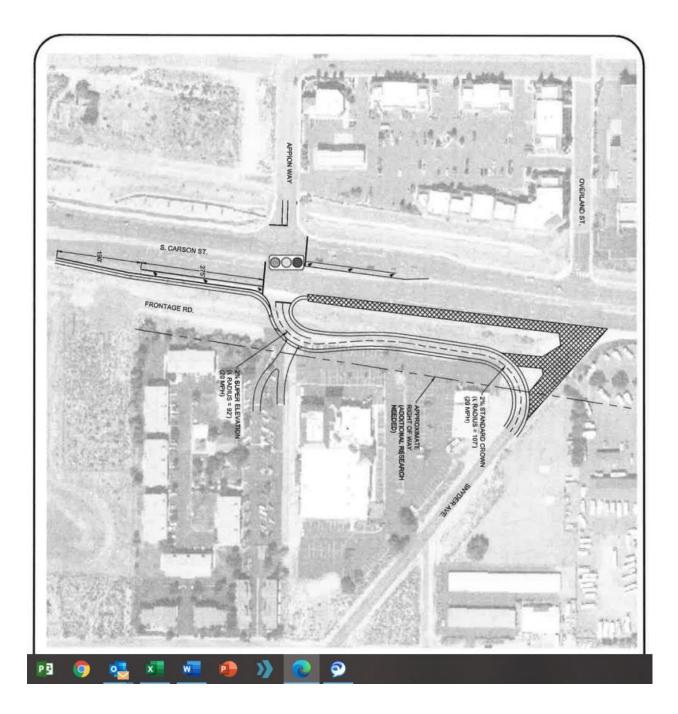
Option 2a of Snyder/Appion alternatives analysis in the southwest Carson City circulation study (not included in final design for construction but to be used as preferred option for conceptual design as basis for intersection geometry)
